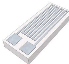
8. Structure after removal of photo-sensitive resist
