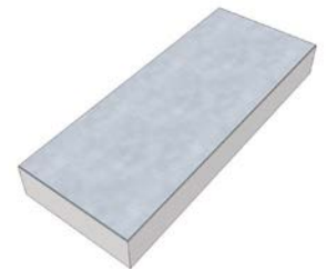
4. Ceramic substrate with thin film metallic layer
